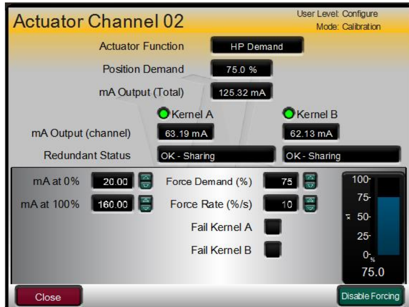
Figure 3-18. Forcing Mode for a Proportional Driver
